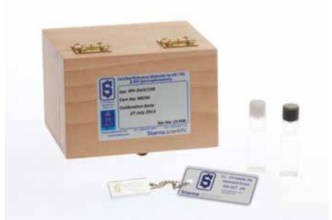
To allow users flexibility in use the reference is supplied with certified wavelength and absorbance values at two different bandwidths, 1.0 nm and 5.0 nm. Nominal values are given below.
