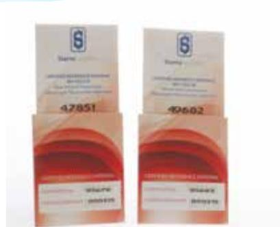
The alternative version has a film thickness of  $65 \mu\text{m}$  and in addition to the peaks listed above, also has certified peaks in the Near-Infrared, covering wavelengths from  $3000 \text{ cm}^{-1}$  to  $9.000 \text{ cm}^{-1}$  ( $3.3$  to  $1.1 \mu\text{m}$ ).
