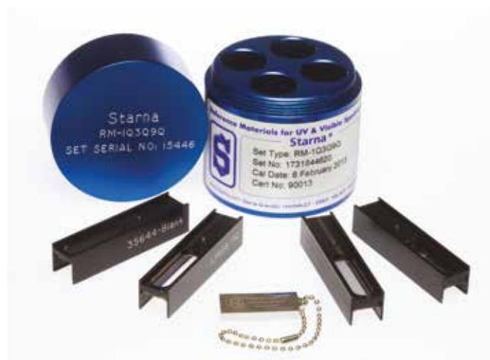
The references are also available individually. Nominal certified transmission/absorbance values and catalogue number are given below. Starna absorbance references are calibrated at a bandwidth of 1 nm. Other bandwidths may be available on request. Any combination of references can be ordered as a set by combining the catalogue numbers as in the example above. An empty filter holder is supplied with each reference or set of references to be used as a measurement blank.
